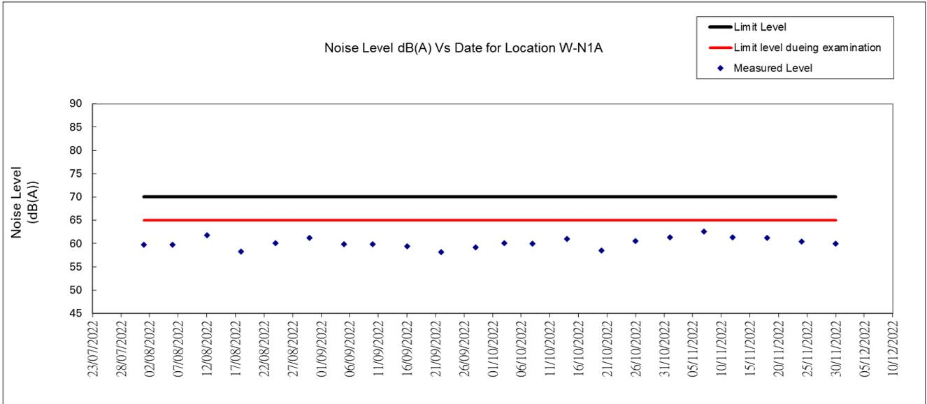
Figure 1: Graphical Illustration of Measured Noise Levels at W-N1A
