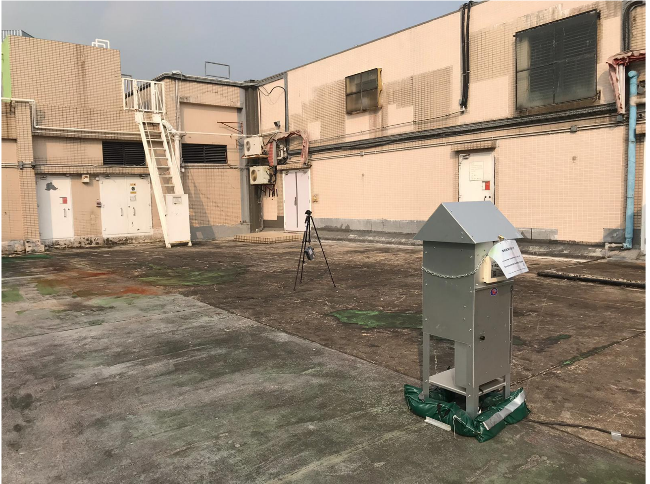
Figure 4.2: Set-up of measurement for 1-hour and 24-hour TSP
